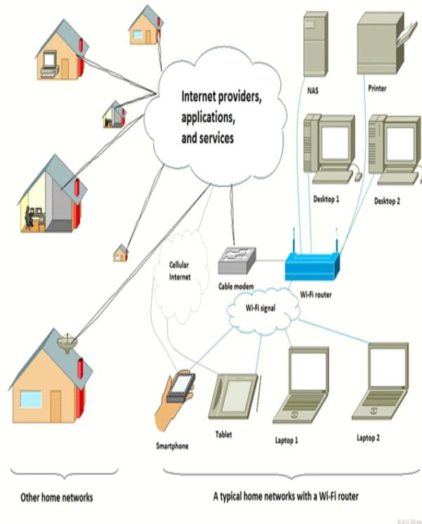
As we can see each and every Wi-Fi signals needs a Wi-Fi router to send and receive data. These routers are again connected by wires to the internet provider through a modem. Wi-Fi works with the help of radio waves and so far every device that gets connected to the internet we need to provide and additional piece of hardware that could send and receive RF signals.
